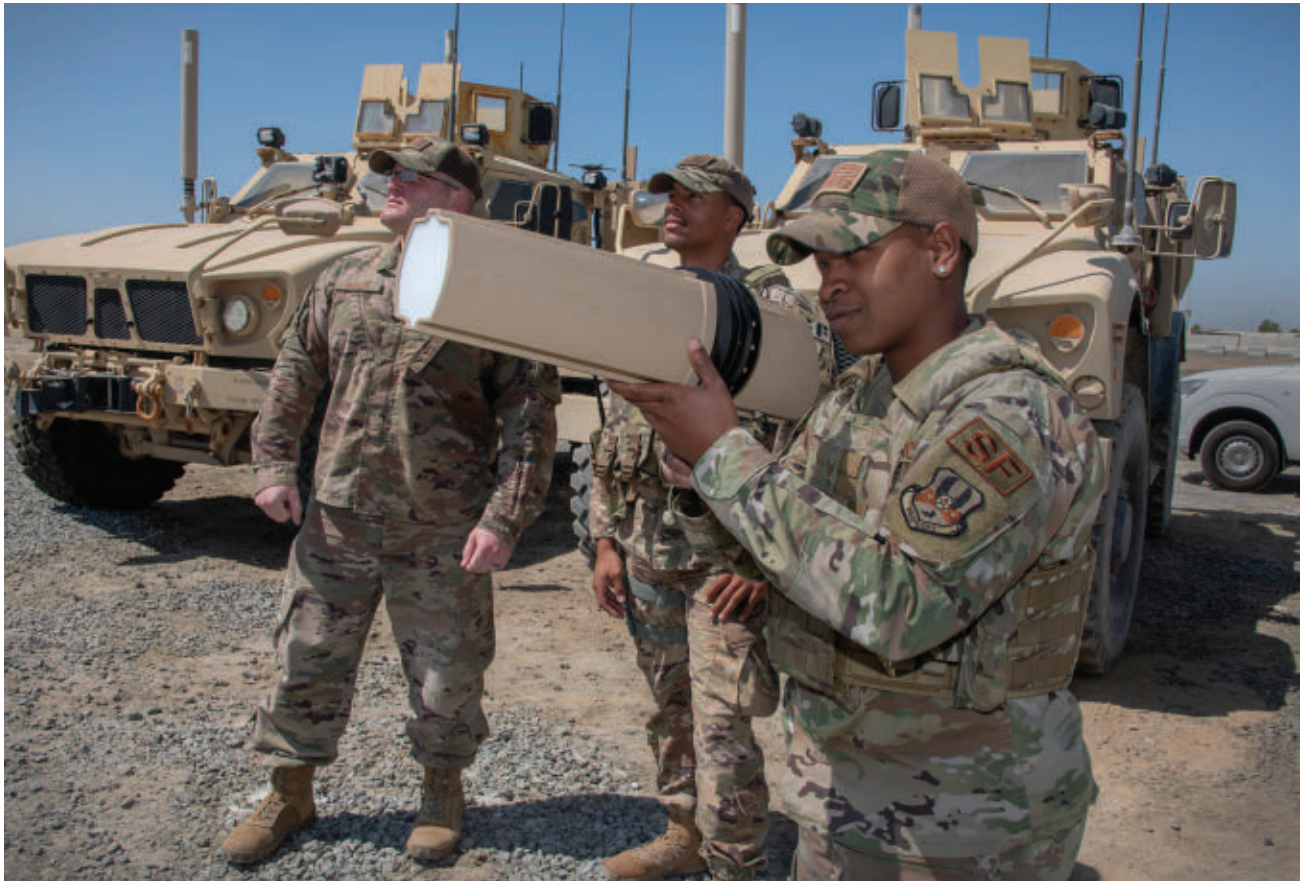
Members of the 380th Expeditionary Security Forces Squadron demonstrate an RF and microwave GPS signal jammer to counter small unmanned aerial systems on Al Dhafra Air Base in the United Arab Emirates.
