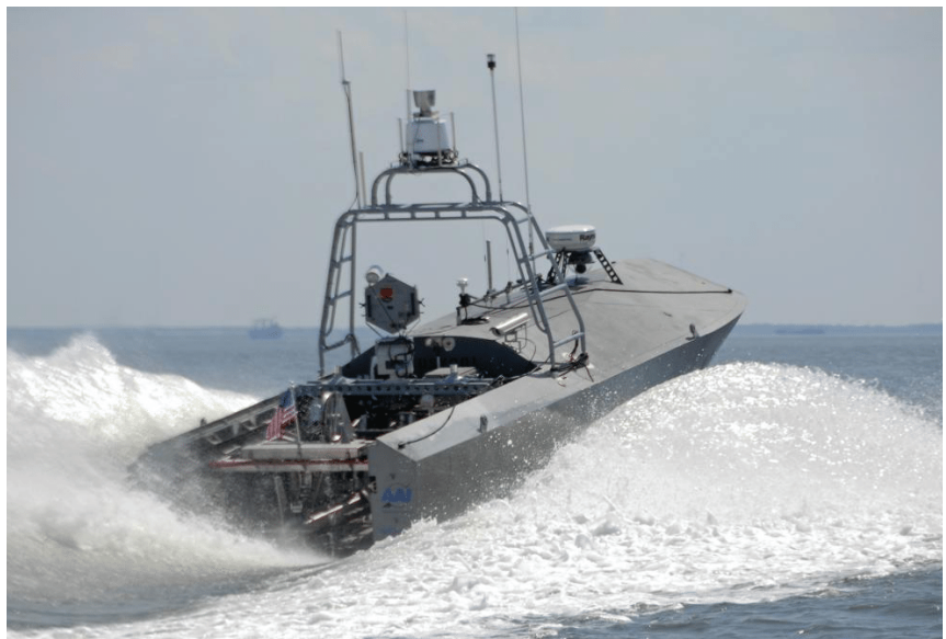
The Mine Countermeasure Unmanned Surface Vehicle (MCM-USV) — a long endurance semi-autonomous diesel-powered aluminum boat — is a prime candidate for new minesweeping sensor payloads.
